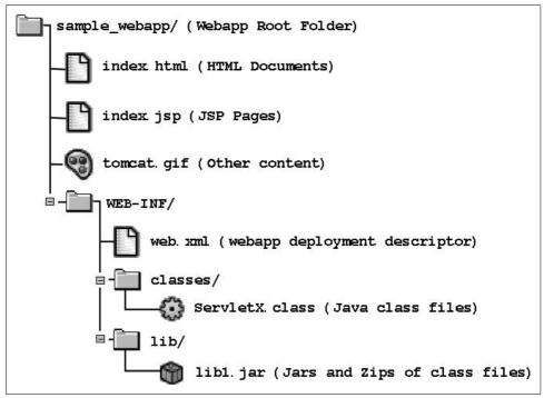
Figure 3-2. Servlet/JSP web application file layout
