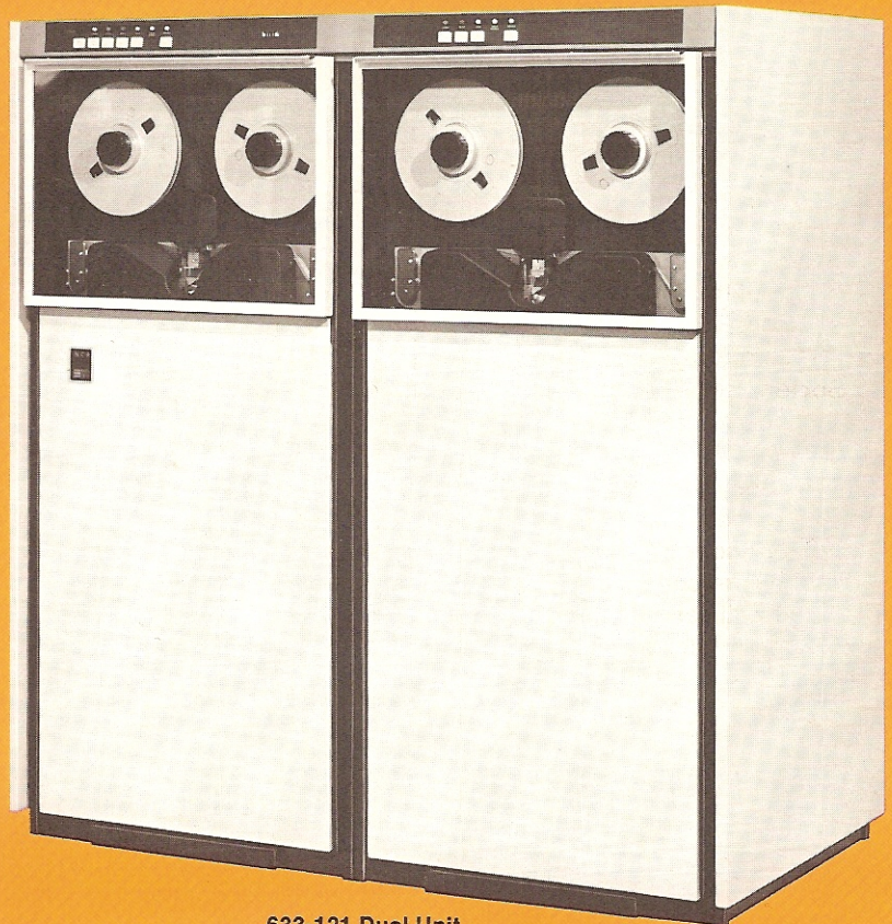
633-121 Dual Unit Magnetic Tape Handler
